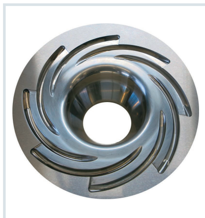
Fig. 1. The circular distribution principle: left: a circular distributor, right: the simulation of radial circumferential distribution after pre-distribution of the melt (© ETA)
